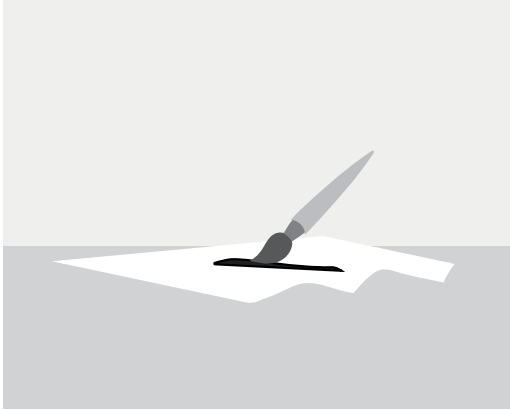
18. Test the colour of the paint before cutting to check that the colour is correct.
